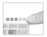
You will then be able to read the degree of water hardness from the discolouration of the Aquadur<sup>®</sup> test strip and the description on the packaging.
